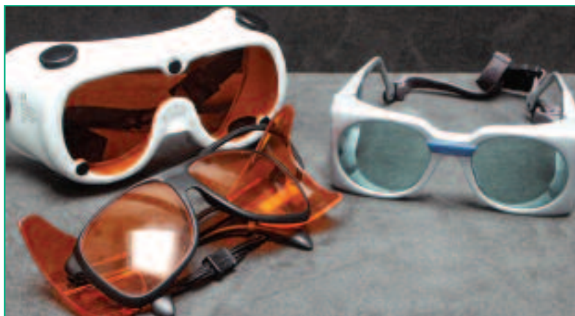
Figure 8 Protective eyewear is available as goggles (which fit over spectacles worn to correct eyesight) or spectacles. The type of lens and level of protection required will depend on the specifications of the laser being used including wavelength, pulse length, maximum pulse energy, repetition rate and beam divergence. Changing from work at one wavelength to another will usually require changing the protective eyewear also.
