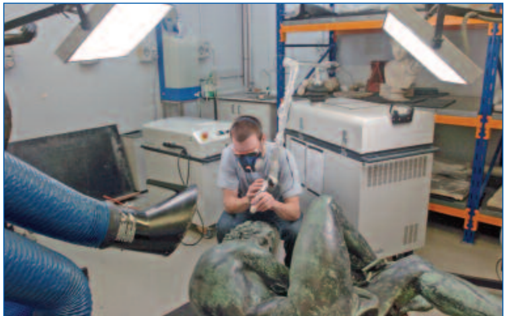
Figure 12 Laser cleaning. The conservator is wearing protective eyewear and a face mask and the waste generated during cleaning is removed by a portable extraction unit.
