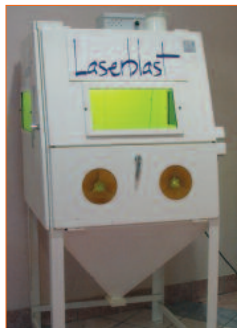
Figure 6 Class I arrangement for laser cleaning. Laser cleaning, using a class 4 laser, is carried out within a glove box so that the laser beam is confined within the box.
